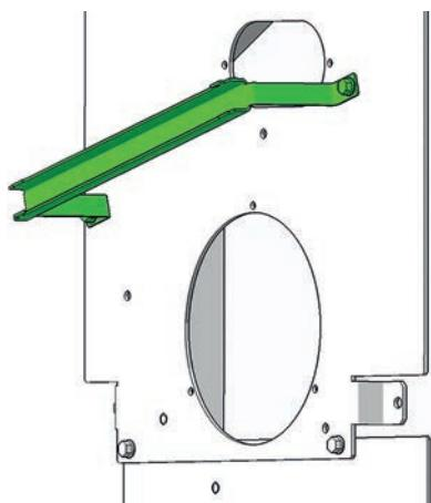
Mount the cable channel again after screwing the second convection fan.
