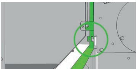
Run the cables between the here shown transparent supply air duct and the conveyor trough back to the green marked vertical cable duct.
