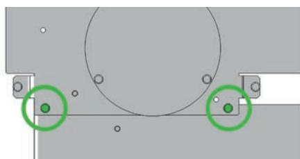
Loosen the screw of the flame sensor. Remove the flame sensor and the silicone hose from the pressure pipe as well.
