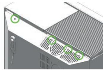
Depending on the desired option cut off the two upper markers for one fan, for the second fan in addition the two bottom markers.
