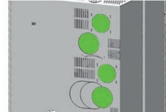
The pre-assembled fan unit must be disassembled for installation. Loosen the screws and remove the entire fan housing with motor and the oval sensor cover. Remove the cable cover which is secured with cable ties.
