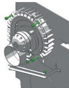
Now mount the lower air deflector on the support plate of the fan.
