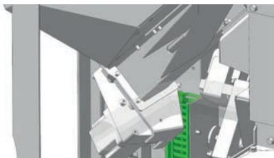
Loosen the nut and the ring from the capacitor till the end from the thread.
